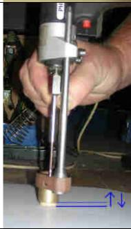
Now try in welding position to lift again by hand, here you should lift the insulations pin 1 to 2 mm. See pic. Below.
