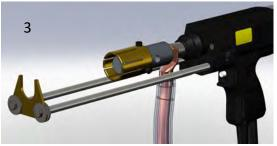
pistol includes a clutch assembly with a tilting ring. What this means in practical terms is that not only can the lift can be adjusted within its operational limits, should certain parameters change from weld to weld, for example the studs being welded varying in length slightly, the pistol will be able to allow for this without affecting the lift that has been set. Even so, we recommend that only properly manufactured weld studs be used to ensure repeatable weld quality.
