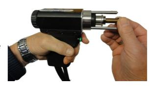
Tighten the chuck locking nut with the box spanner provided. A gentle pressure is all that is required. Over tightening may result in damage to your pistol.
