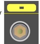
Connect the welding pistol control cable to the controller. Note that the cable end plug and panel mounting socket are keyed to prevent incorrect fitting. Push the plug firmly home and twist the locking ring clockwise to secure the plug in position.
